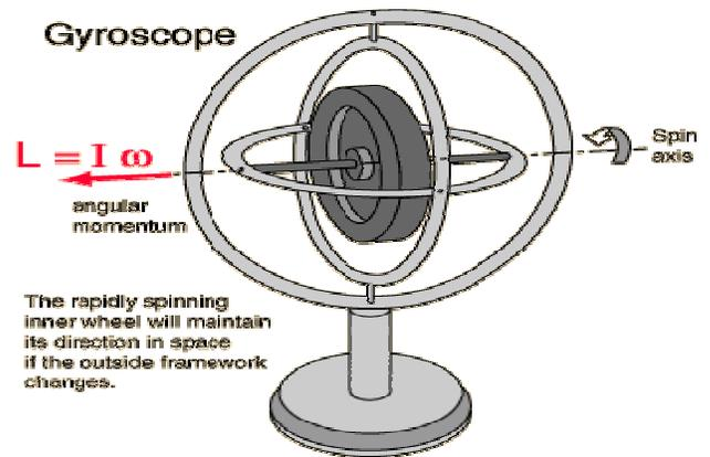
**Fig. 2:** A gyroscope: its structure and function
