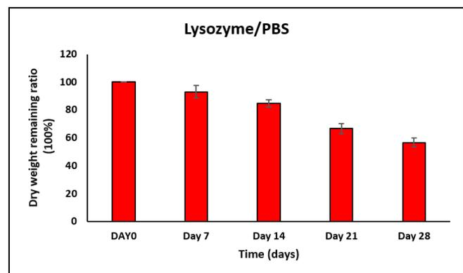
**Fig. 6:** In vitro degradation in PBS and Lysozyme. We managed to mimic the physiological environment by selecting two media for degradation; PBS and lysozyme. From the results, it was concluded that
