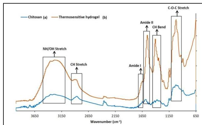
Fig. 2: FTIR results of pure chitosan (a) and thermosensitive hydrogel (b).
