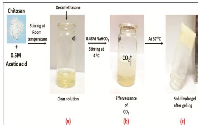
Fig. 1: Step by step illustration of synthesis of thermosensitive hydrogel.
